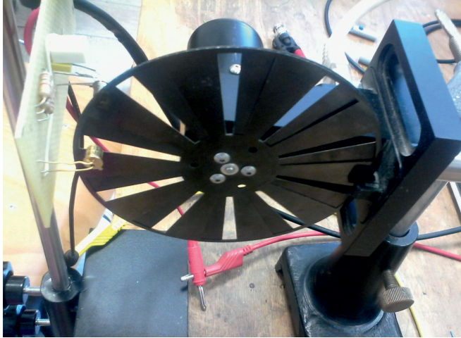
Figure 3.10: A classical chopper, used to test the response of the used laser diode and photodetector.
