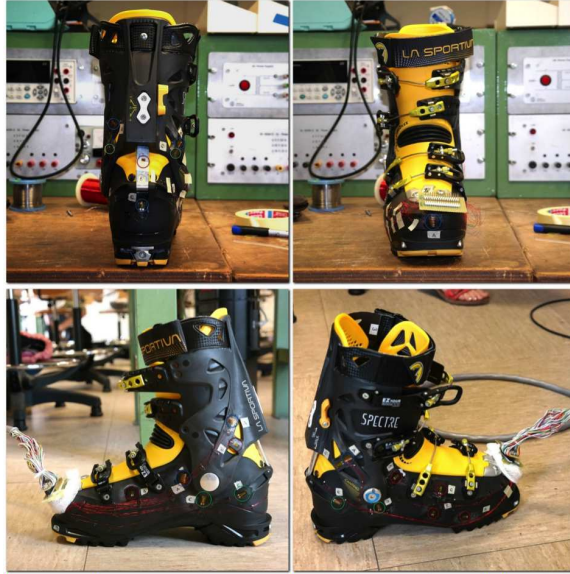
Figure 2.5: Gauges location on a ski-boot specimen.
