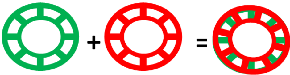
Figure 3.13: Relative dephasing of the bladed wheels varies the aperture and therefore the duty cycle of the optical signal, maintaining the same frequency.
