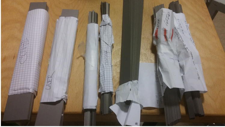
Figure 2.7: The laminated iron samples
