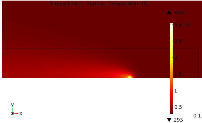
Figure 2.17: Thermal distribution in the sample at a fixed time. The brightest spot indicates the position of the laser.
