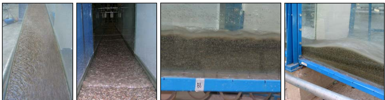
Fig. 1: from left to right: alternated bars, roll waves over mobile bed, antidunes moving downstream and antidunes moving upstream in the channel.
