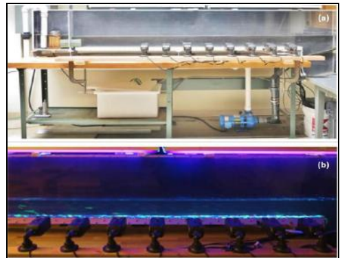
Figure 1. Experimental set-up of the Plexiglas flume (top) and installed series of 8 synchronized video cameras recording travel paths of fluorescent painted particles under black light (bottom), after Naqshband et al. (under review).
