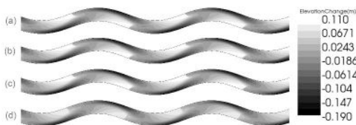
Figure 1. Elevation change from an initially flat bed, for the channel with crossing angle \omega = 20^\circ . (a) - (c) are from the unsteady flow run ((a) Q_w = 0.026 m 3 /s, (b) Q_w = 0.07 m 3 /s, (c) Q_w = 0.13 m 3 /s) and (d) is from the constant-discharge run ( Q_w = 0.07 m 3 /s).
