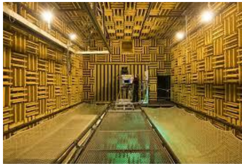
Anechoic wind tunnel LMFA, Centrale Lyon
