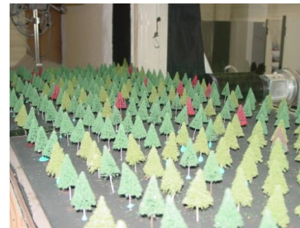
Tree canopy in wind tunnel IRPHE, Centrale Marseille
